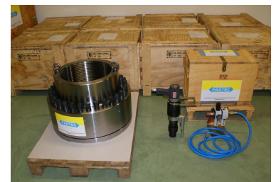
mechanical tensioner for press columns Ø450
